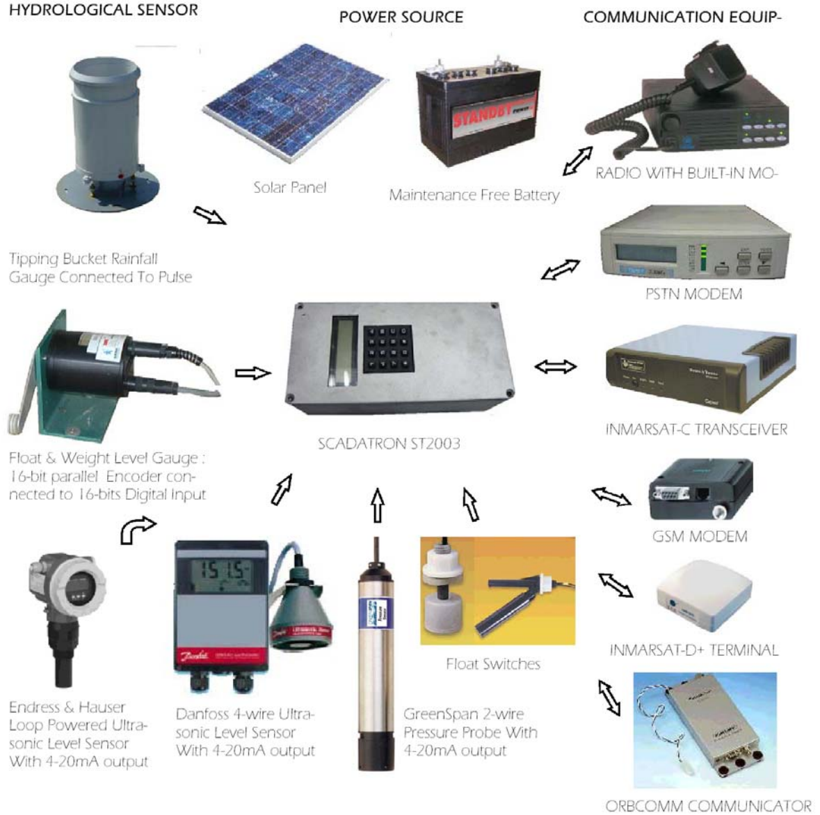
Diagram above shows some of the sensor instrument and communication equipment able to connect to ST23 RTU
