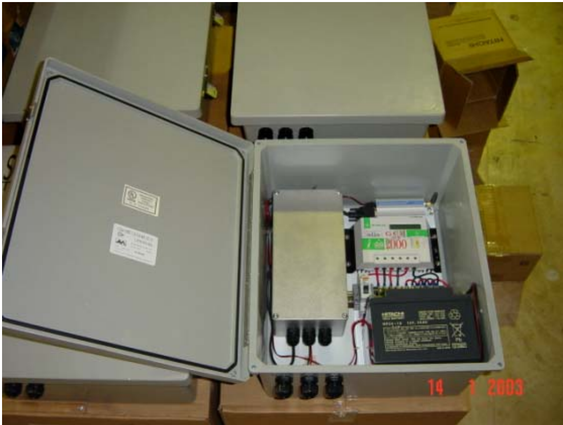
A Scadatron Telemetry ST23 Remote Terminal Unit when placed in a NEMA-4X Enclosure
