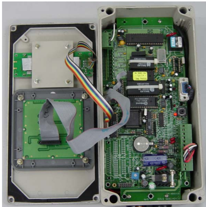
Internal view of ST23 RTU
