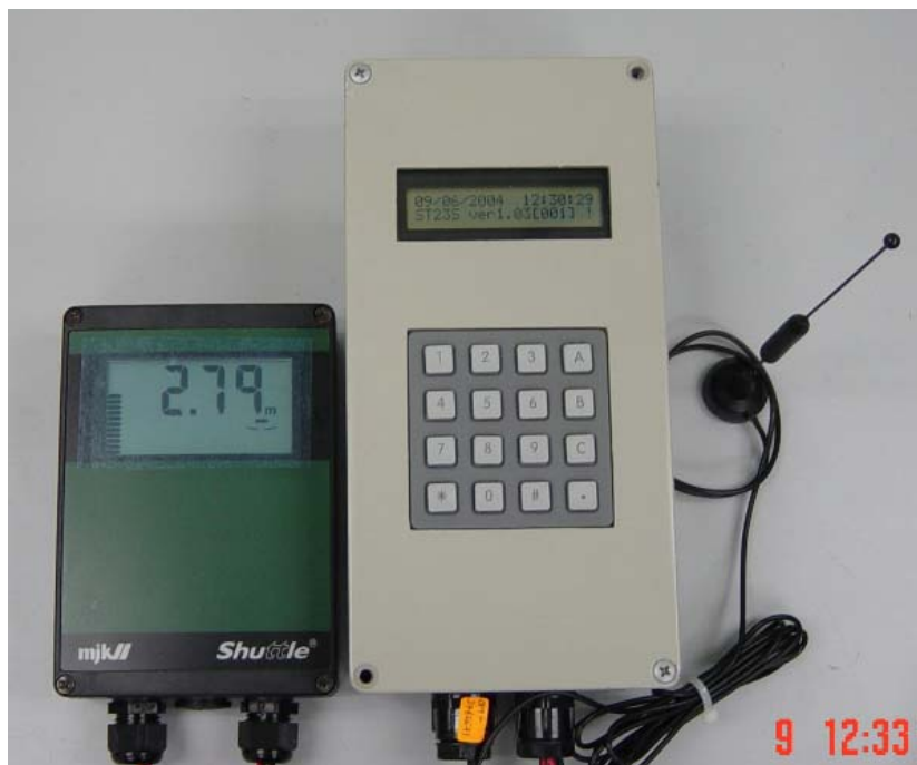
External view of ST23 RTU with a typical ultrasonic water level transmitter
