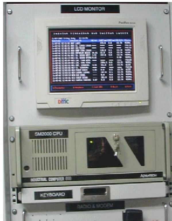
Detail view of the SM2000 FEP Industrial Computer 19" rack and LCD display panel displaying alarm / event / data with time stamp
