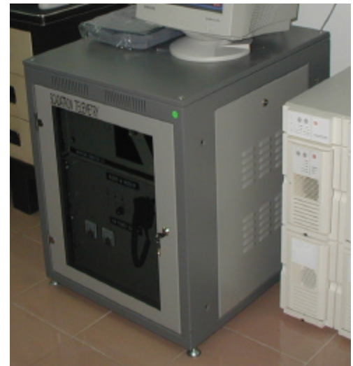
FEP in a 13U height 19" Equipment rack
