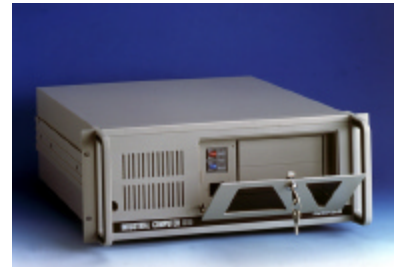
A FEP implemented using Industrial graded PC for reliable operation
