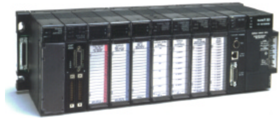
A GE-Fanuc PLC with power supply module, CPU module and some Input/output modules on a back-plane
